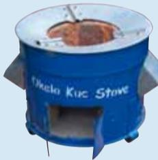
**Energy Saving Stoves** have a metal outer jacket and a thick clay inner layer. The clay acts as an insulator, reducing the amount of heat lost. It also increases the amount of heat being transferred to the cooking pot, so food cooks faster.
